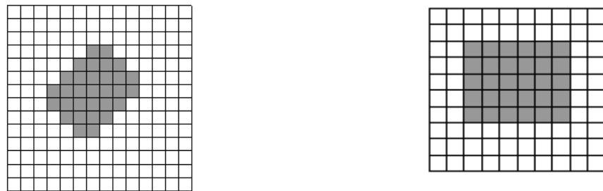
Figure 4 Original MIKE SHE grid (orientation = 315°), and after converting to ArcView (orientation = 0° or N-S).
